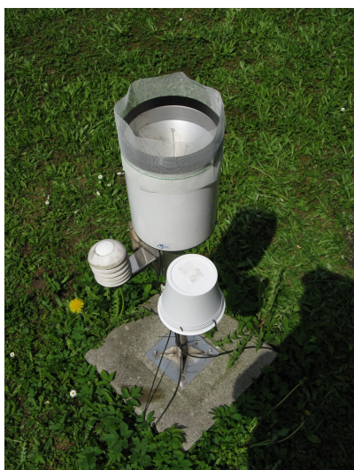
(a) Stojan meteostanice
